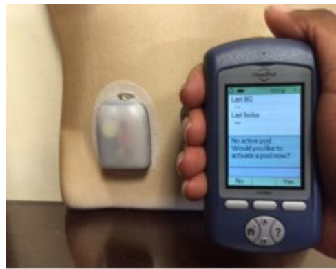
Figure 3: The OmniPod tubeless insulin pump with a pod( right) and hand held device that functions as a blood glucose meter and communicates wirelessly with the pod to deliver insulin based on the patient's personal settings.
