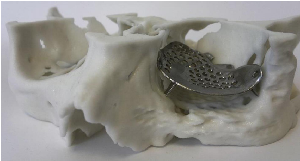
Figure 2: The rapid prototype metal orbital floor reconstruction in the orbit of the stereolithic skull reconstructed from the original CT scans (Keyhan et al., 2016)
