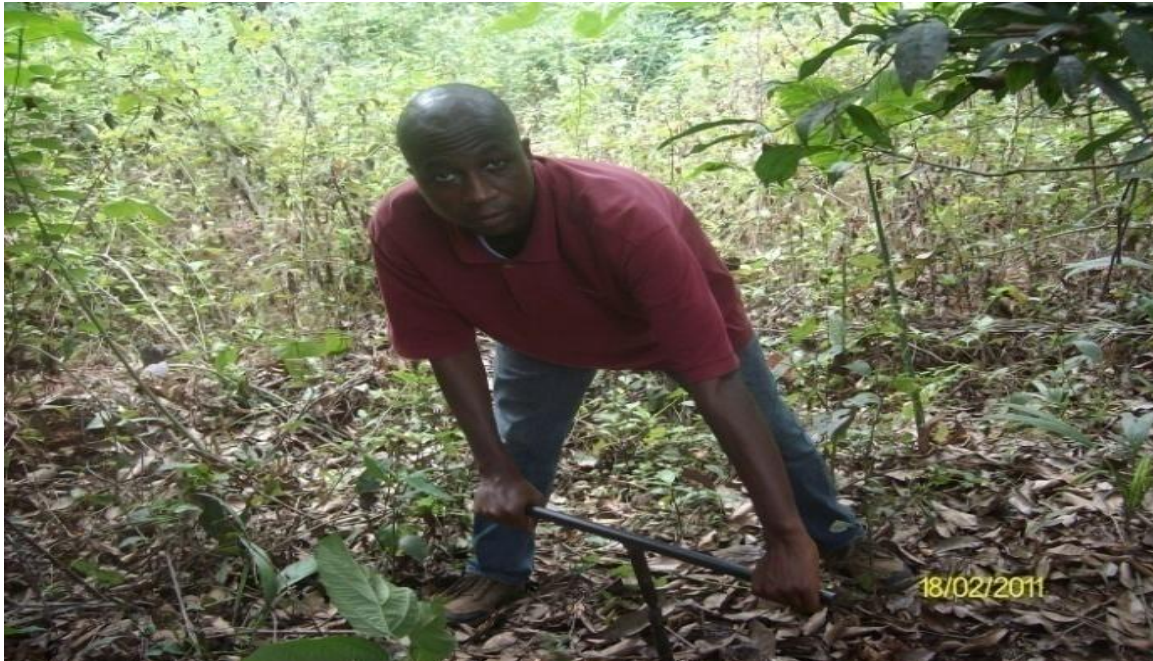
Plate 1: Samples were collected with the use of a hand auger.
