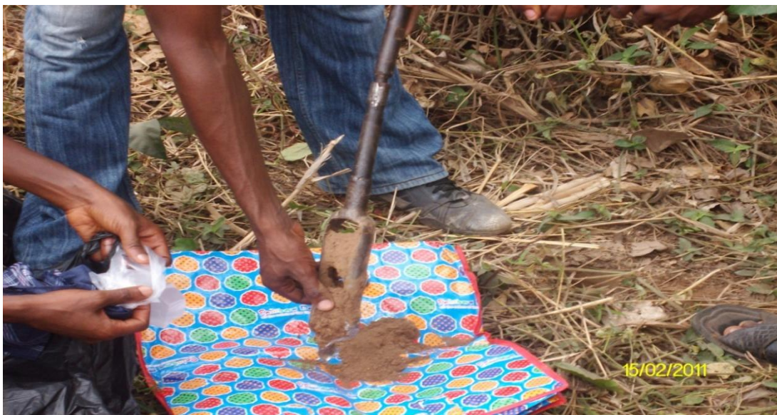
Plate 2: Several pinches of samples collected with a hand auger were well-labelled and stored in a sample bag.
