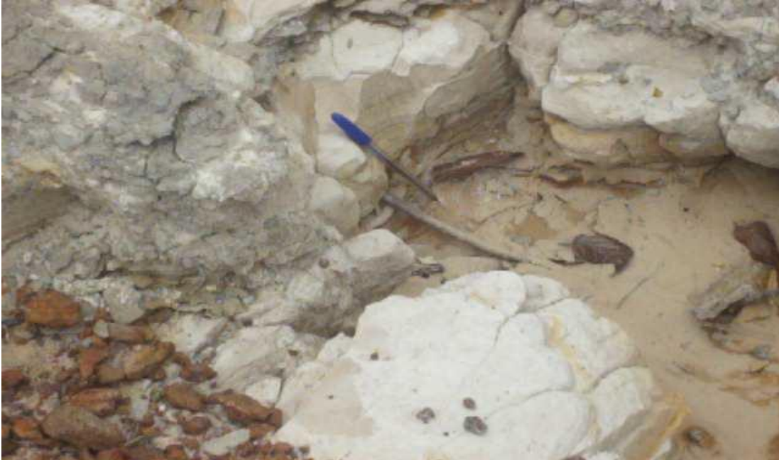
Plate 3: Weathered shale sample exposed at Lokpanta. The shale is hard, light to dark grey and fissile.
